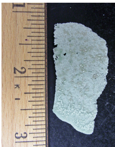
This is one of the samples after 10 minute exposure to cleaner "A." This product was only minimally effective at dissolving the sample.
