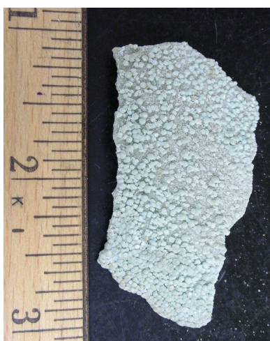
One of two identical scale samples used in a scale cleaner efficacy study to determine which cleaner would remove the scale most effectively.
